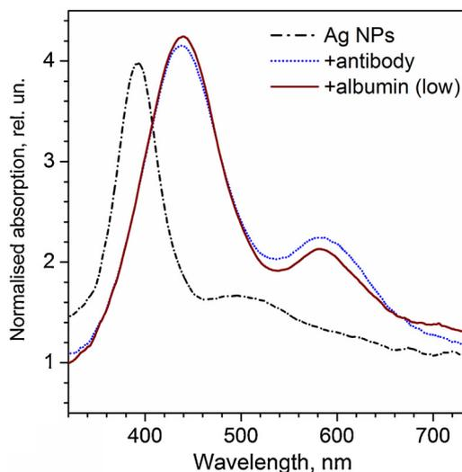
**Fig. 6.** Normalised optical absorption spectra of quartz substrates with as-deposited clusters followed by antibody-antigen incubation scheme (anti-chicken egg albumin antibody followed by chicken egg albumin). Albumin concentration is reduced for six times compared to the case presented in Fig. 5.
