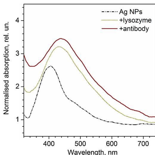
**Fig. 8.** Normalised optical absorption spectra of quartz substrates with as-deposited clusters followed by inverted antigen–antibody incubation scheme (lysozyme followed by anti-chicken egg albumin antibody).
