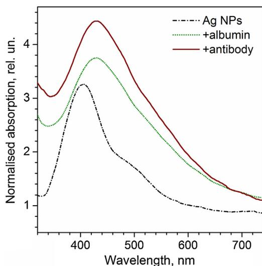
**Fig. 7.** Normalised optical absorption spectra of quartz substrates with as-deposited clusters followed by inversed antigen-antibody incubation scheme (chicken egg albumin followed by anti-chicken egg albumin antibody).
