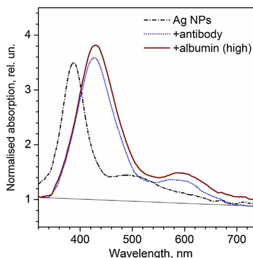
**Fig. 5.** Normalised optical absorption spectra of quartz substrates with as-deposited clusters followed by antibody-antigen incubation scheme (anti-chicken egg albumin antibody followed by chicken egg albumin). Straight base line is shown for one of the spectra.
