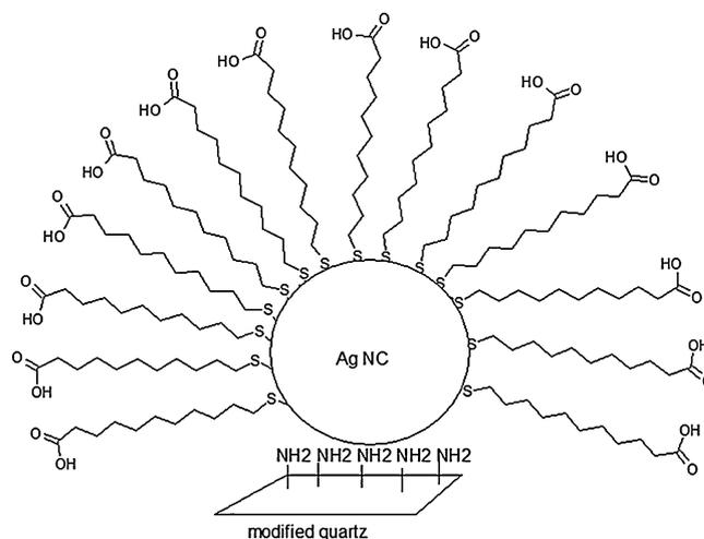
Fig. 2. Functionalisation of silver cluster surfaces using 11-MUA.
