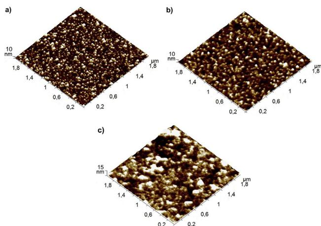
**Fig. 4.** AFM images of substrates (a) with as-deposited clusters, (b) after antibody-antigen incubation (classical scheme) on clusters and (c) after antigen-antibody incubation (inverted scheme) on clusters.
